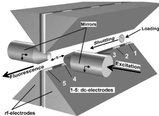
**Figure 1.** Setup of the single-ion CQED system used in the experiment. The loading zone and the cavity interaction region are located at opposite ends of the linear trap. The rf electrodes are shaped to provide optimum side access for laser beams and placement of the cavity mirrors.
