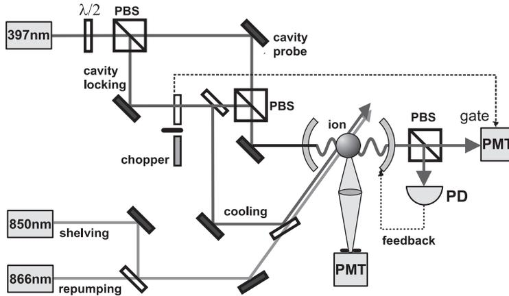
**Figure 4.** Setup of the laser system used for locking the cavity and exciting and diagnosing the ion coupled to the cavity field. The laser at 850 nm is used for shelving the ion in the  $D_{5/2}$  state.
