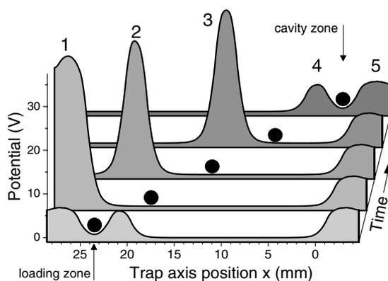
**Figure 2.** Sequence of axial potential distributions used to shuttle the ion from the loading to the cavity zone, obtained from a three-dimensional finite-element calculation. The black circle indicates the position of the ion, the electrode numbers correspond to those in figure 1.
