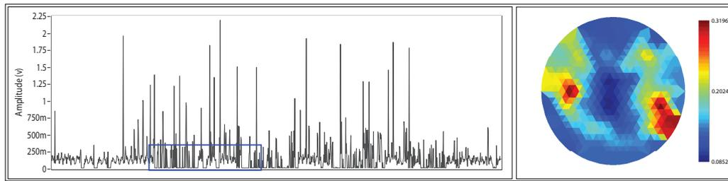
**Figure 2.** The breast scan shows clear signs of saturation that dominate the back-projection image. In the highlighted area, significant numbers of measurements were at 0V, effectively non-measurements.
