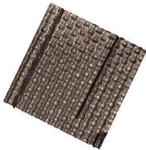
Figure 3. 3-D rendering of surface potential with an excitation signal of 100 kHz. Two linear surface defects may be seen in addition to the internal structure of the material.
