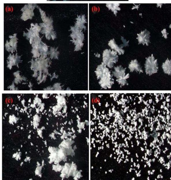
**Figure 1.** Optical microscopic image of agglomerates made of IPA, a: SLS, b: tween, c: PVP, d: HPMC.
