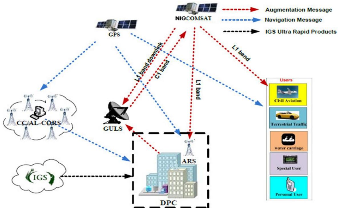
Figure 9: Nigerian Satellite Augmentation System Architecture.
