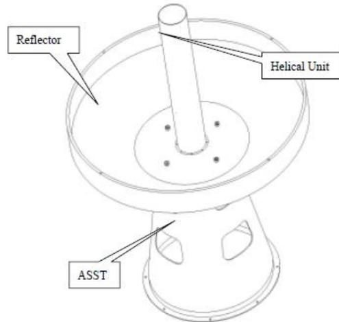
Figure 4: Helical L-Band Navigation Antenna Structure Configuration
