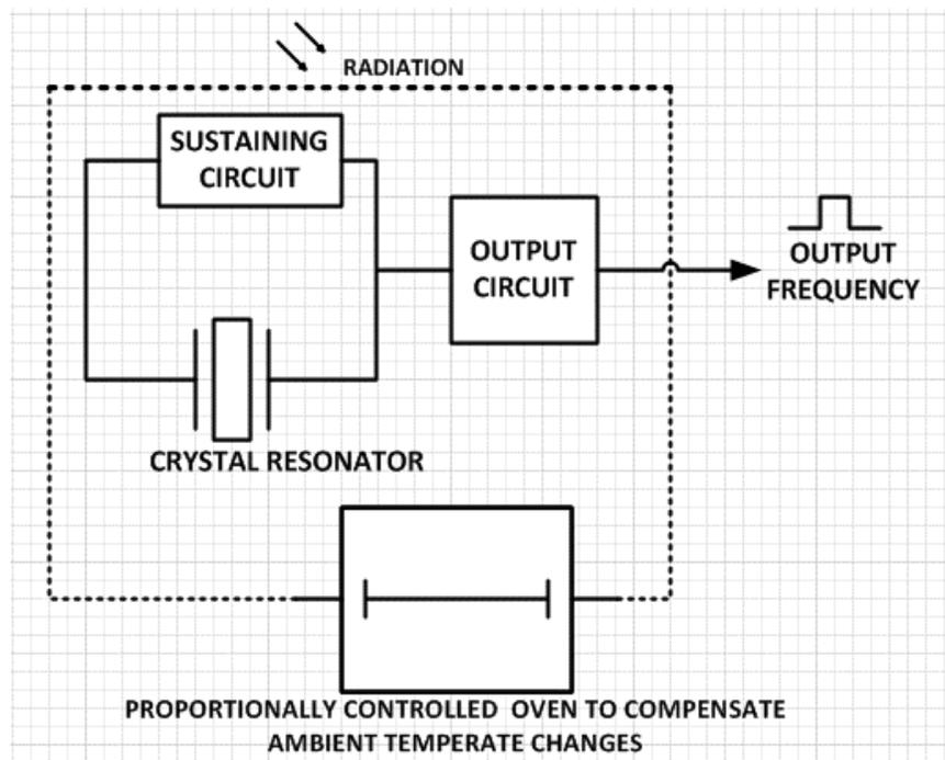
Figure 5: A Typical Ovenized Crystal Oscillator (OCXO) showing its Crystal Resonator and external circuits in a proportionally controlled oven to compensate ambient temperature changes.
